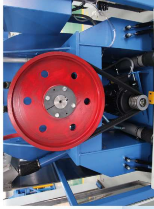
Simple and efficient direct v-belt drive system
