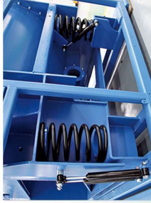
Robust springs and shocks suspension system for vibration free operation
